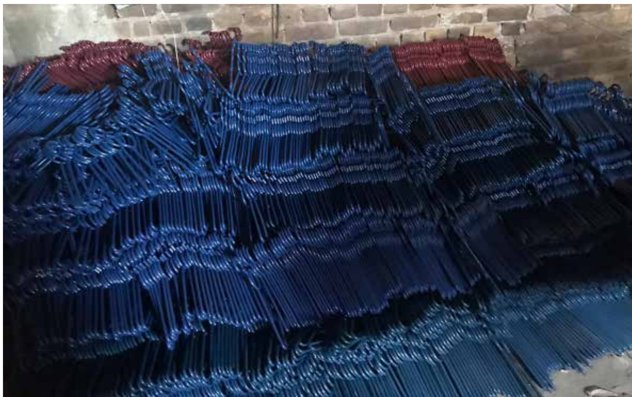
Figure 113: PET crushed and made into hangers by a recycler
