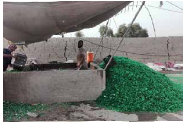
Figure 130: Flakes of crushed PET bottles being washed, Rahim Yar Khan
